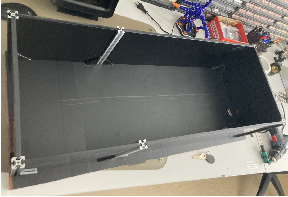
Figure A.4: Picture of the self build optical enclosure (black box) from the inside
